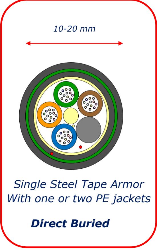
General Backbone Cable - Buried
